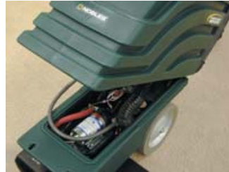
The clam-shell design on the Power Eagle™ and Frontier™ extractors allow for quick and easy access to components.
