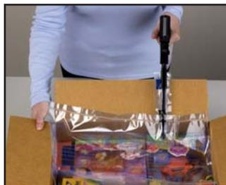
2. Insert the inflator nozzle into the Fill-Air® RF bag and place the bag on top of products.
