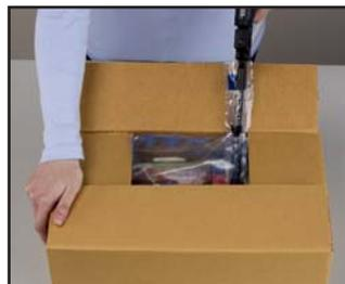
3. With carton flaps partially closed, fill the bag until the void is filled. The clear bag allows for a visual check.
