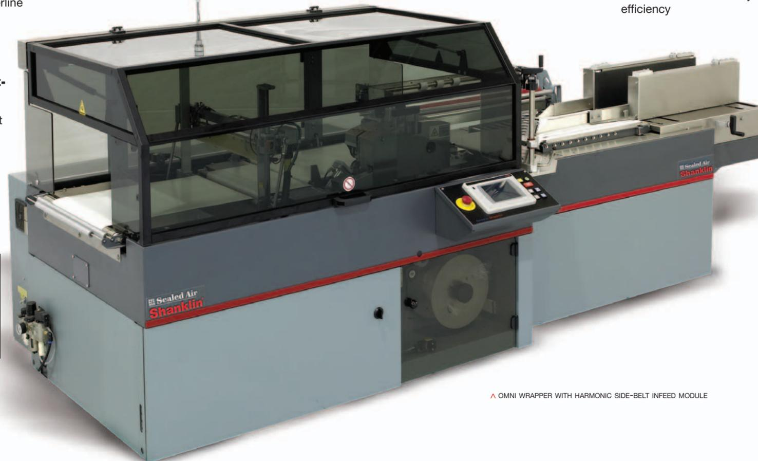
▲ OMNI WRAPPER WITH HARMONIC SIDE-BELT INFEED MODULE
