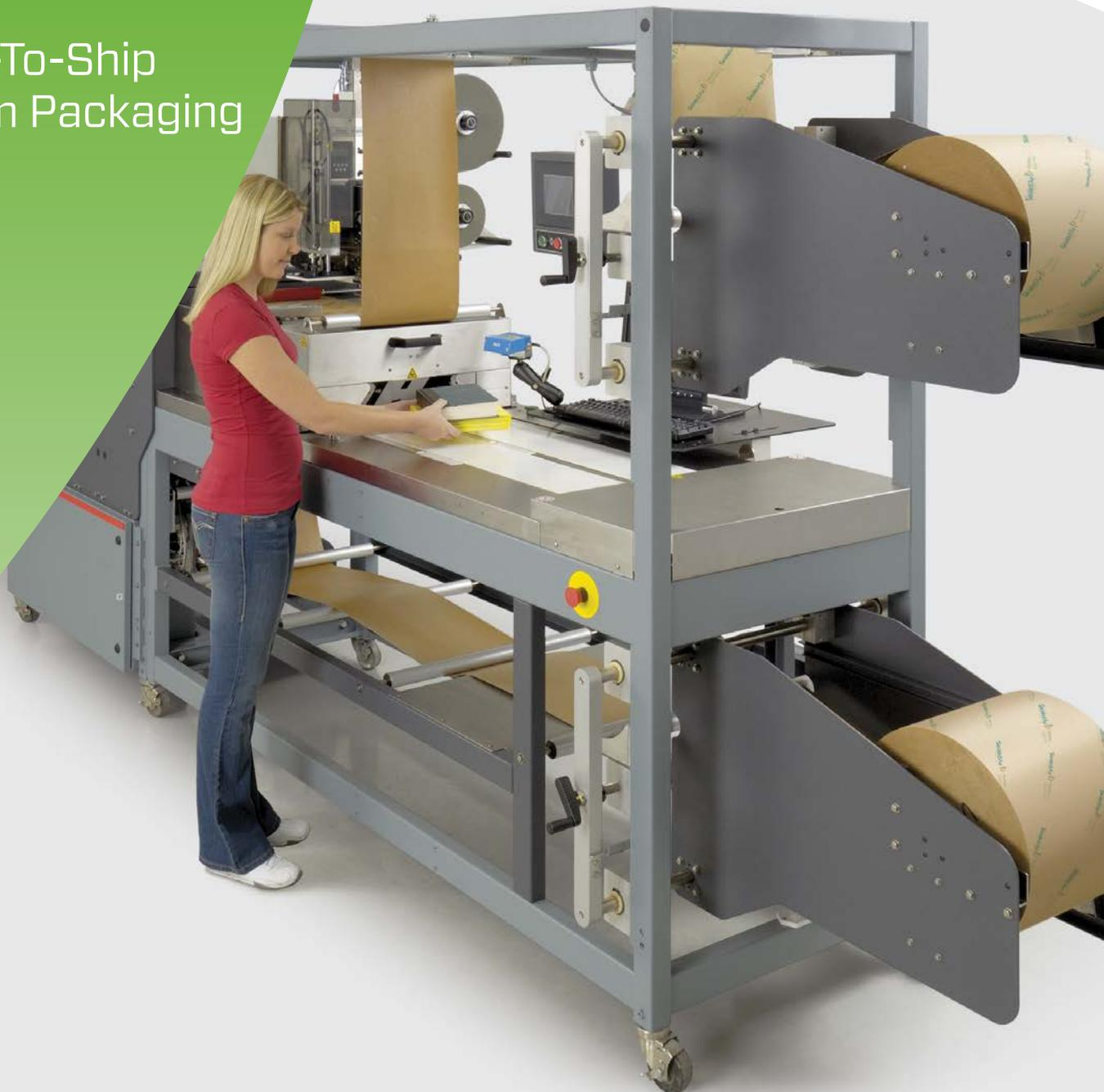
The PriorityPak® system shortens the packaging process and maximizes your use of labor by creating up to 15 packages a minute, compared to only 1–3 packages a minute when using manual packaging methods.
