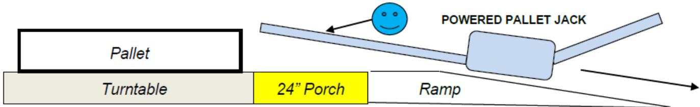
When do you need the optional porch? In most cases a porch is not necessary when using a standard manual pallet jack. It may be necessary when the machine is being loaded with a powered pallet jack, a “ride-um” or any other larger specialized material handling equipment.
